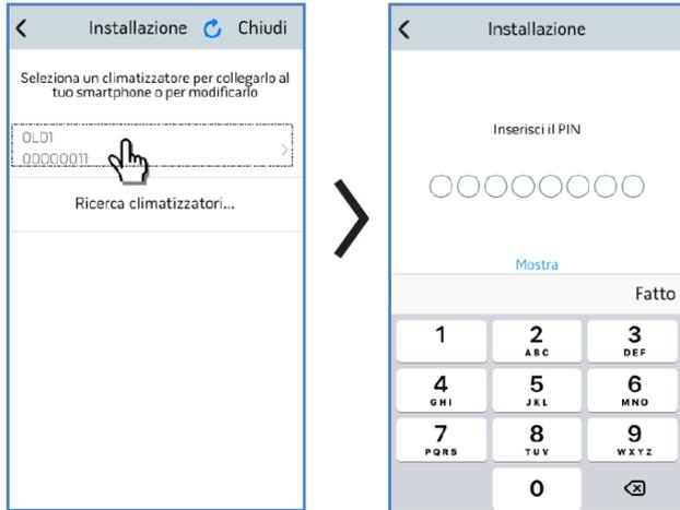
ATTENTION: The pin cannot be modified. It is unique for each kit B1015, so it must be kept with care for any new recordings of the air conditioner on the app. It is therefore suggested to apply one of the labels provided in the kit near the machine data plate
