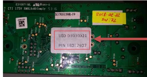
The UID and PIN references are also shown on the back of the electronic card.
