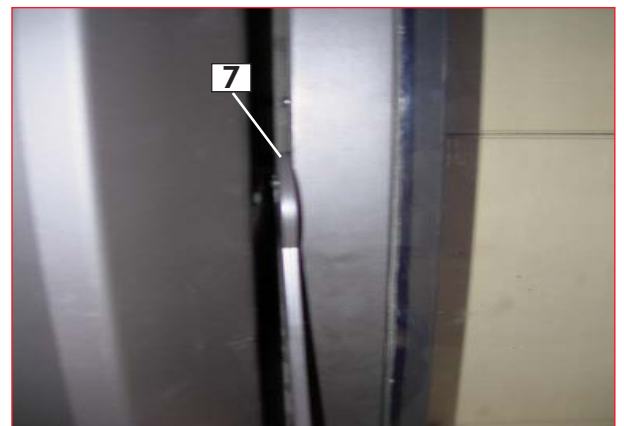
Figure 3 : blocking the door open (rotate the pawl by 90°)
