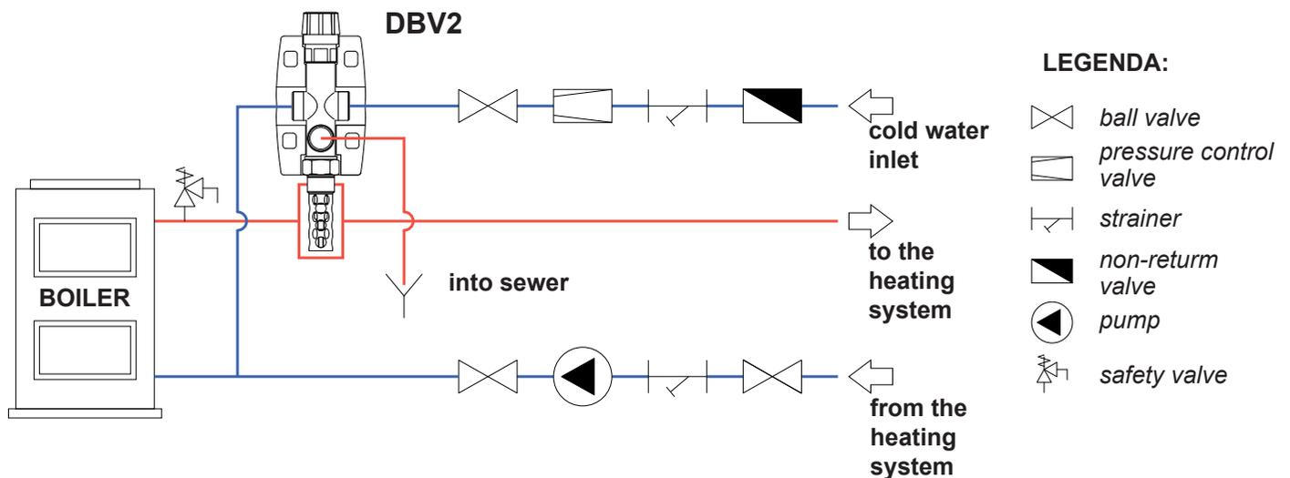
Fig. 3: Piping diagram for DBV2
