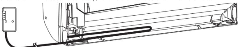
Run the connecting cable in the space on the back of the unit as shown in the above figure.
