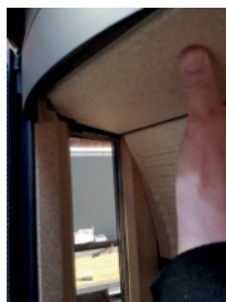
2: The top baffle plate is carefully lifted over the two vermiculite posts in front of the stove.
