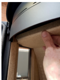
1: The top baffle plate is to be pushed up into the front.
