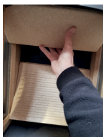
5: The top baffle plate can now be removed.
