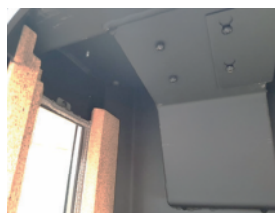
6: Loosen the 4 Allen screws with a 4mm Allen key. See Photo 6a. The metal baffle plates 1 and 2 can now be slightly pushed back and can then be removed. The stove is now ready for cleaning.
