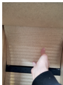
3: Once the top baffle plate from instruction 2 has been lifted, the upper vermiculite back plate can be lifted across the tertiary beam.
